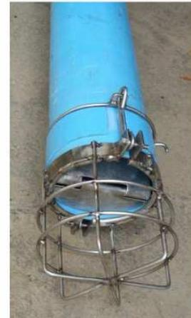
Figure 3 - Strainer and valve at the bottom of the riser pipe
